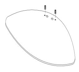
Place the Threaded Posts in the Base inside the corners of the Cover (P4).
