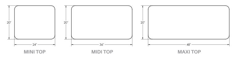
\*\*Laminate tops are 1 1/8" thick particle board core with HPL and 3mm T-mold Edge\*\*
