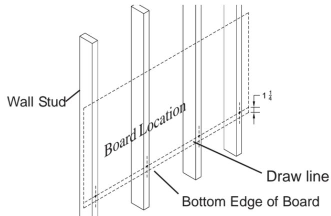
**1** Determine board location. Measure from floor to the bottom edge of board. Mark with pencil line the corner location. Measure up from bottom edge of board 1-1/4" and draw line as shown. Locate stud near each end of board and drill pilot holes along line using 1/8" drill bit. See diagram below.
