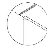
**3** Set board on the Angle Brackets. Draw line along top edge of board.
