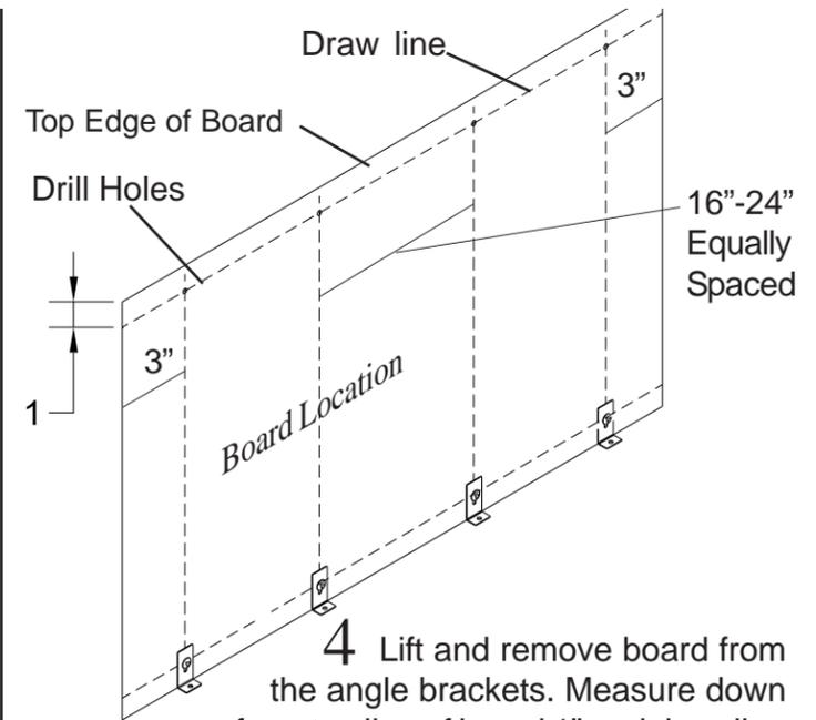
**4** Lift and remove board from the angle brackets. Measure down from top line of board 1" and draw line as shown. Locate stud near each end of board and drill pilot hole along line using 1/8" drill bit.
