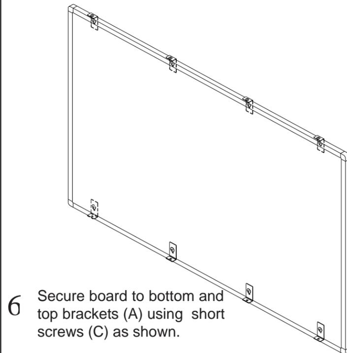
**6** Secure board to bottom and top brackets (A) using short screws (C) as shown.
