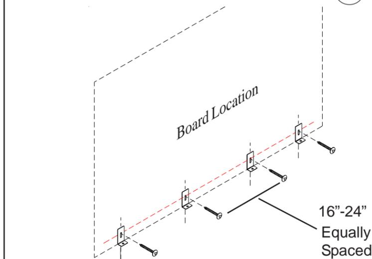
**2** Attach 1/2 the # of Angle Brackets using Long Screws (B) as shown.
