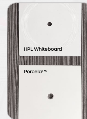
In-house Taber testing shows porcelain steel has superior resistance to abrasion.
